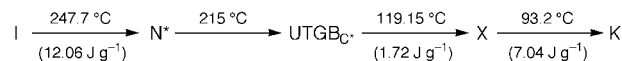
Scheme 2 The number in parenthesis indicates the transition enthalpy; X is a highly ordered mesophase and yet to be fully characterized; K = crystal.
