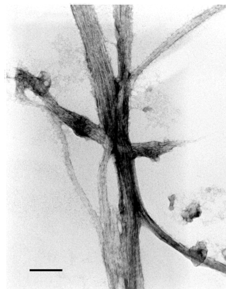
Fig. 18 Transmission electron microscopy image of poly(phenolformaldehyde) mesofibers extracted from poly(phenolformaldehyde)-mesoporous silica composite. Scale bar = 10 nm.
