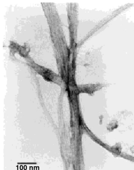
Fig. 25 A TEM micrograph of polymer mesofibers formed by polyaddition/condensation of phenol and formaldehyde within the mesoscopic channels of MCM-41. Reprinted in part with permission from: J. Mater. Chem. , 1998, 8, 13 (© 1998, The Royal Society of Chemistry).
